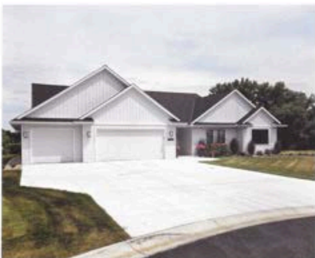
10" Board & Batten Seamless Steel Siding in Glacier White 5" Horizontal Seamless Steel Siding in Glacier White
