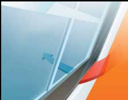
Diagram B – Warm Edge Spacers block heat escape paths.
